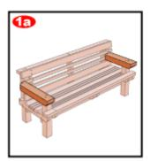
b Trim the front end of each 4x6 armrest at a 45-degree angle, beginning one and one half inches down from the top. Make a 3 1/2-inch square notch in the inside back of each armrest where it will wrap the rear leg, and finish with a 45-degree bevel cut.
